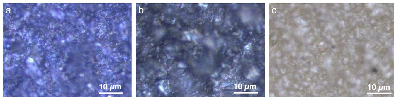
Fig. 1. Optical micrographs of (a) IrO<sub>2</sub>, (b) RuO<sub>2</sub>, (c) ITO thin films on Al<sub>2</sub>O<sub>3</sub> substrate.
