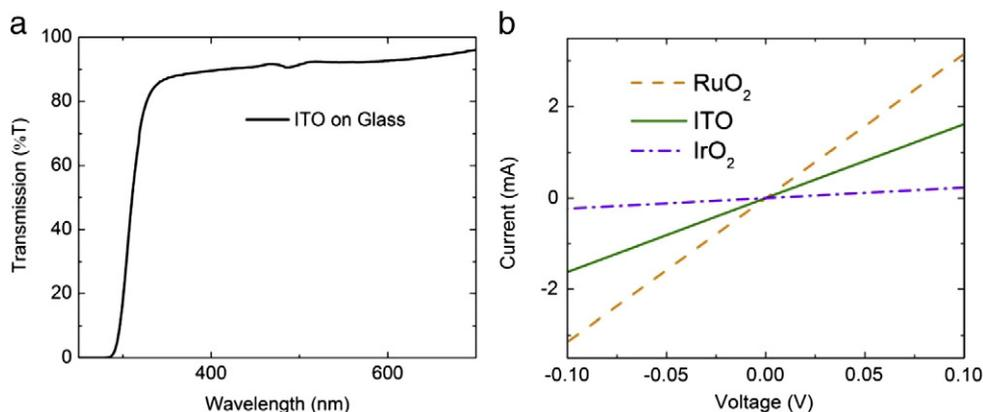
Fig. 3. (a) Optical transmission of 300 nm ITO film deposited on a glass "sister" sample. (b) Current–voltage characteristics of IrO<sub>2</sub>, RuO<sub>2</sub>, and ITO thin films on Al<sub>2</sub>O<sub>3</sub> substrates.
