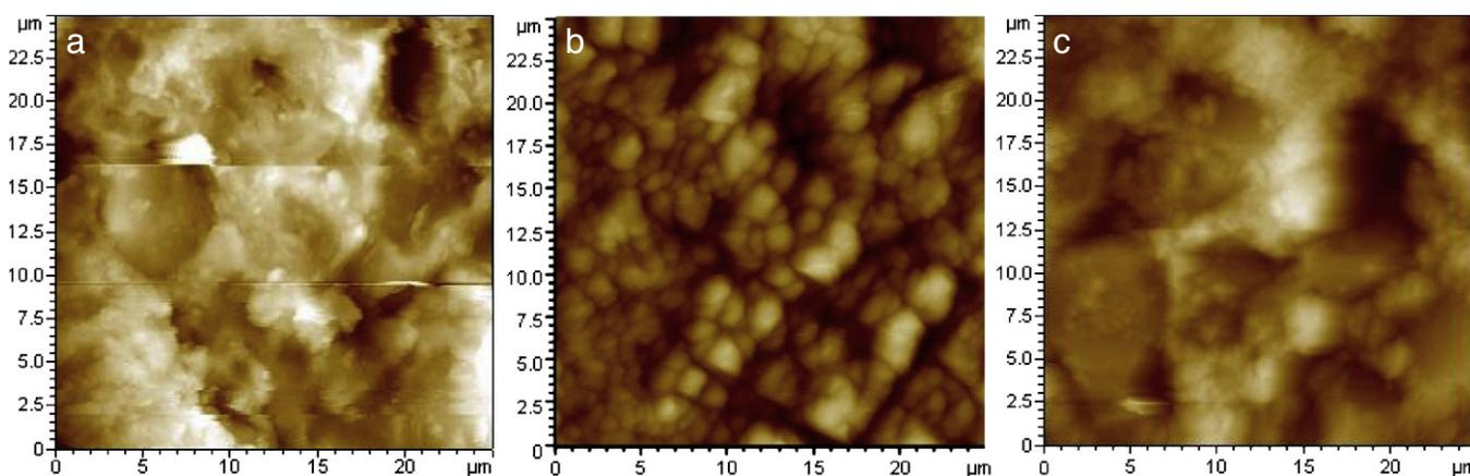
Fig. 2. AFM surface images of (a) IrO<sub>2</sub> (scale: 0 to 3000 nm), (b) RuO<sub>2</sub> (scale: 0 to 7000 nm), and (c) ITO (scale: 0 to 1500 nm) thin film layers deposited on Al<sub>2</sub>O<sub>3</sub> substrates.
