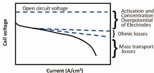
**Figure 10.** Schematic of polarization effects in an operating fuel cell.
