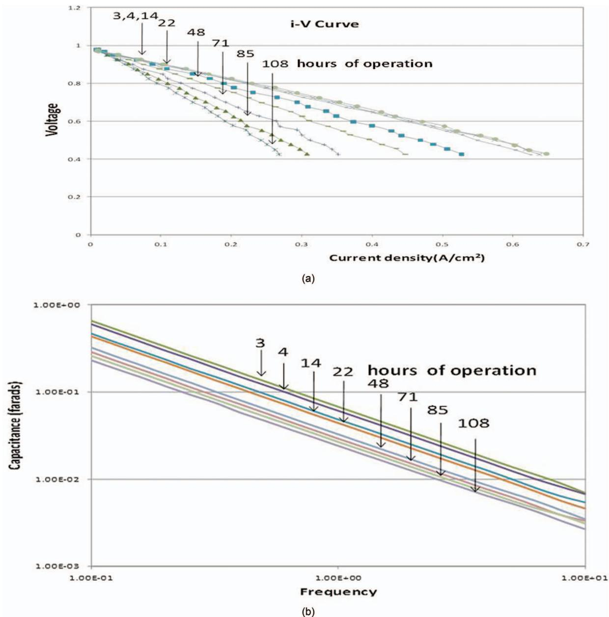
Figure 11. Polarization curve for an SOFC cell (a) measured after several hours of operation, and non-faradaic capacitance measured after each period (b).
