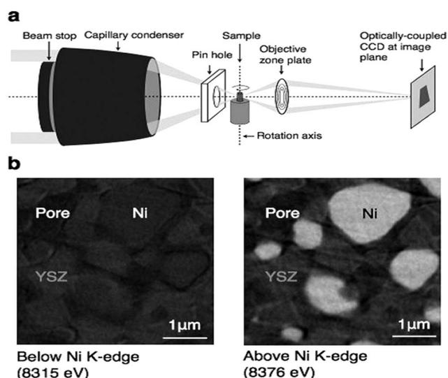
**Figure 4.** (a) Components of transmission X-ray microscope. (b) Illustration of elemental mapping using absorption contrast imaging: slices within the reconstructed XNT data of a Ni-YSZ anode, below and above the Ni K-edge.
