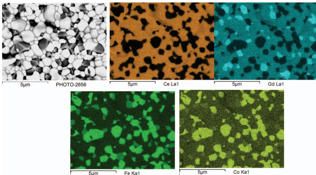
**Figure 7.** 0.6CGO-0.4CFO Sintered at 1300°C for 2 hours SEM-Secondary Electron Image and EDS chemical composition analysis.
