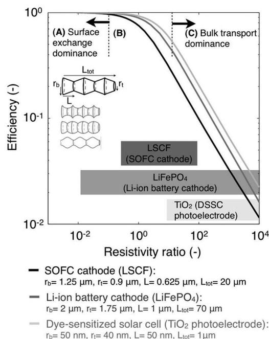
**Figure 14.** Fin efficiency as a function of resistivity ratio for SOFC cathode, Li-ion battery cathode, and dye-sensitized cells represented by periodic assemblies of one profile type for which analytical solutions exist (conical frustums). The grayscale bars indicate the approximate range in resistivity ratio, hence accessible regime, for the typical materials used for these systems.
