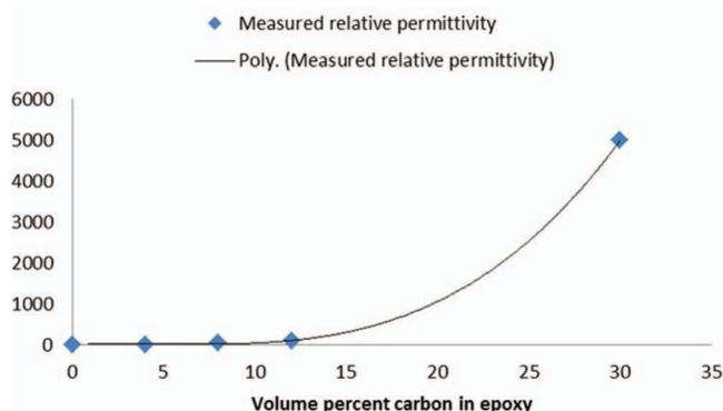
**Figure 13.** Measured composite permittivity of carbon flakes embedded in epoxy matrix for increasing volume percent.
