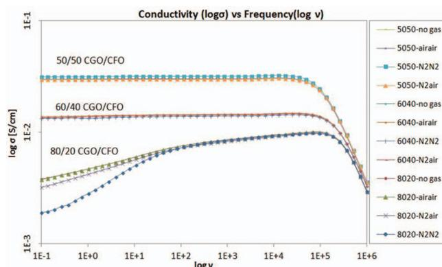
**Figure 9.** BDS Conductivity versus Frequency at various gas flows at 800°C for 50/50, 60/40, and 80/20 volume% CGO/CFO.
