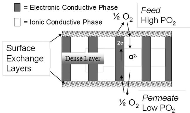
**Figure 6.** Oxygen Separation Membrane: Function and Principle.
