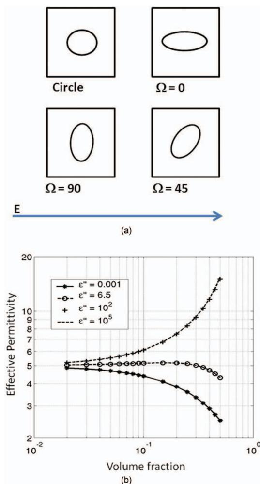
**Figure 12.** Representative volume elements (a) used for the Physalis solution method to determine local charge storage and effective permittivity in non-dilute heterogeneous dielectric materials,<sup>67-69</sup> and HeteroFoaM effective permittivity (at 10 Hz) predicted for different constituent properties (b) showing emergent property characteristics.
