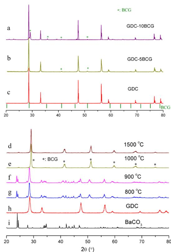
**Figure 1.** XRD patterns for (a) 10BCG–GDC (10%  $\text{BaCO}_3$ ), (b) 5BCG–GDC (5%  $\text{BaCO}_3$ ), and (c) pure GDC pellets sintered at 1500 °C for 5 h. GDC– $\text{BaCO}_3$  composite powder (mole ratio of 50:50) calcined at (d–g) 1500, 1000, 900, and 800 °C respectively, (h) pure GDC powder, and (i) pure  $\text{BaCO}_3$  powder.
