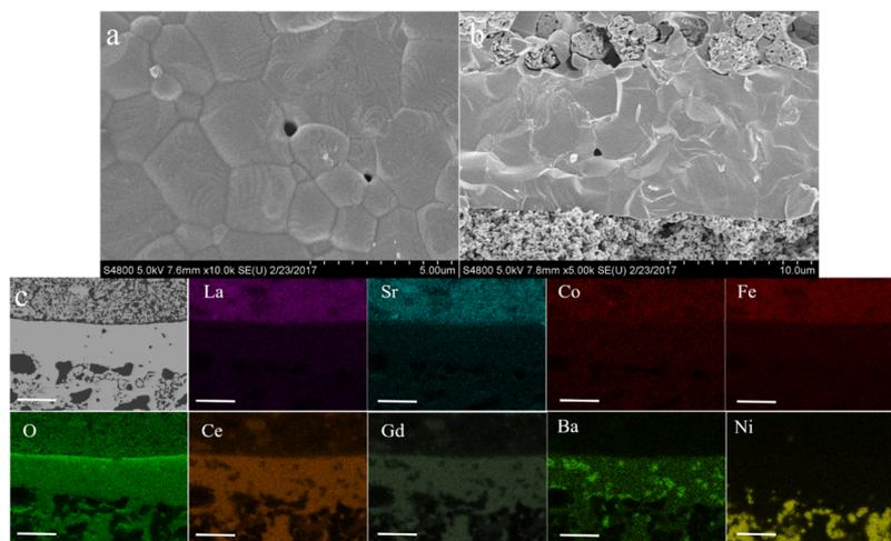
**Figure 9.** (a) Surface area and (b) cross section of the SBCG-GDC electrolyte after 100 h of operation. (c) Backscatter SEM of full cell cross section after the 100 h test and EDX element mapping in BSE mode for La, Sr, Co, Fe, Ce, Gd, Ba, and Ni elements. Scale bars, 10  $\mu\text{m}$ .
