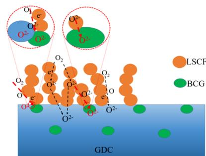
**Figure 7.** ORR mechanism schematic diagram for the LSCF cathode on the SBCG–GDC electrolyte.
