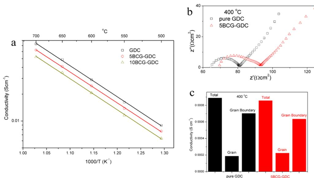
**Figure 3.** (a) Ionic conductivity of pure GDC, 5BCG–GDC, and 10BCG–GDC electrolytes, (b) impedance spectra, and (c) contribution of grain and grain-boundary conductivity at 400 °C.
