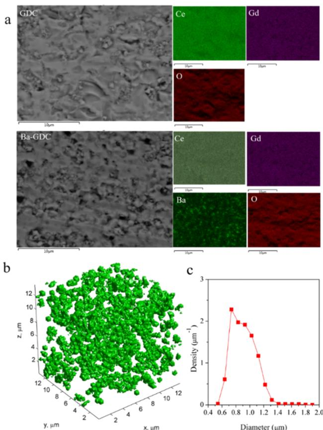
**Figure 6.** (a) SEM–EDX images for GDC and SBCG–GDC electrolytes, (b) 3D distribution image of the BCG phase in the GDC matrix, and (c) grain size distribution of the BCG phase.
