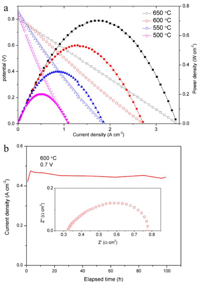
**Figure 8.** (a)  $V$ - $I$  performance of the SBCG-GDC electrolyte full cell with the LSCF cathode and (b) current density with 0.7 V voltage at 600 °C and corresponding ac impedance spectra.
