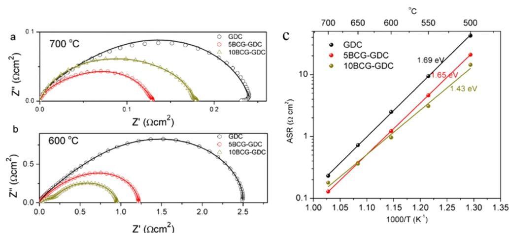
**Figure 4.** (a,b) Impedance spectra of the LSCF cathode in GDC, 5BCG–GDC, and 10BCG–GDC electrolytes at 700 and 600 °C and (c) area specific polarization resistance (ASR) of the LSCF electrode on GDC, 5BCG–GDC, and 10BCG–GDC from 500 to 700 °C.
