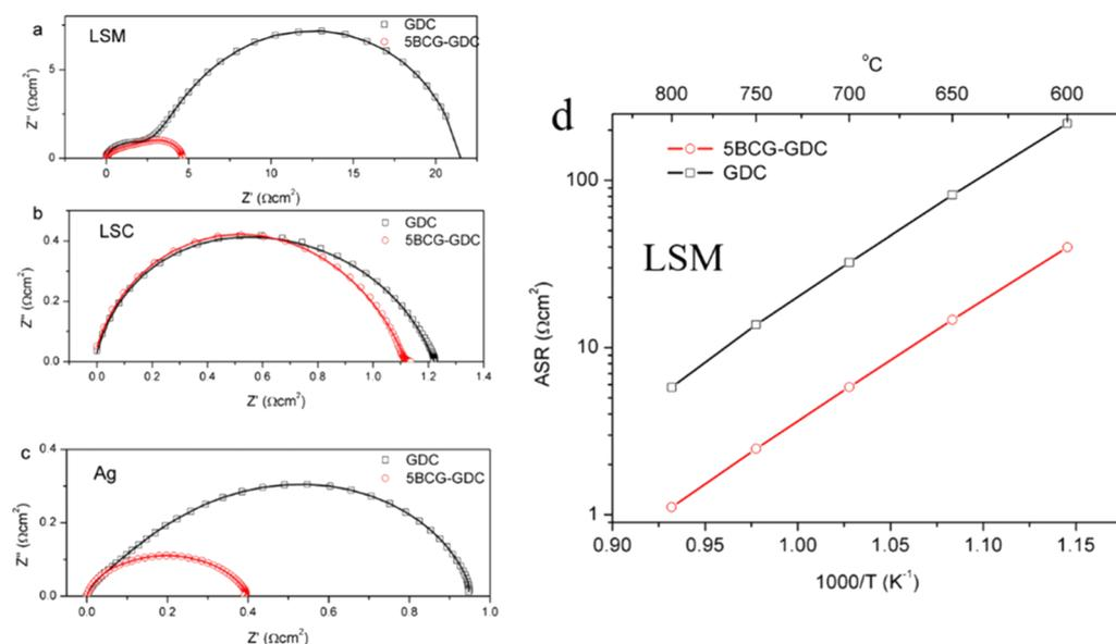
**Figure 5.** Polarization resistance of (a) LSM, (b) LSC, and (c) Ag on GDC and 5BCG–GDC electrolytes at 700 °C and (d) corresponding ASR value of the LSM electrode from 600 to 800 °C.
