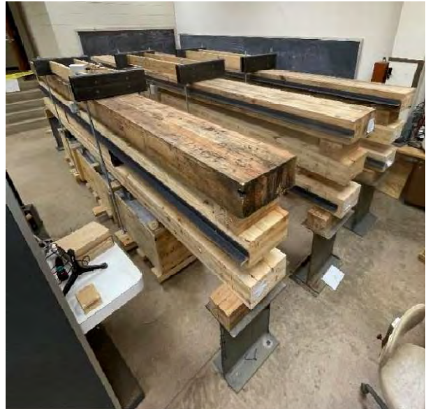
Creep setup with three stacks of CLT and GLT members loaded and instrumented to measure deformation (creep)
