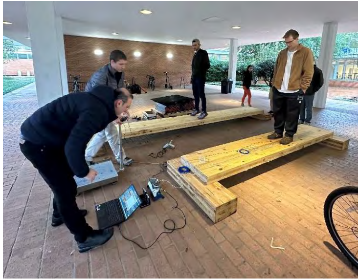
Graduate students participating in experimental vibration measurement of CLT panels
