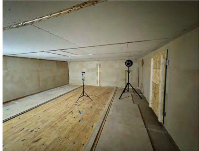
Lifting the experimental timber floor system into place and the subsequent acoustic testing within the two-story test chamber
