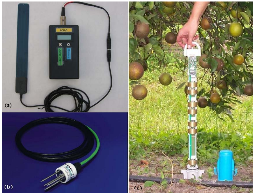
Figure 5. Frequency domain (FD) probes: a) capacitance (plates embedded in a silicon board); b) capacitance (rods); and c) FDR (rings).
