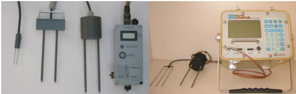
Figure 4. Time domain reflectometry (TDR) equipment showing probe versions and readouts.
